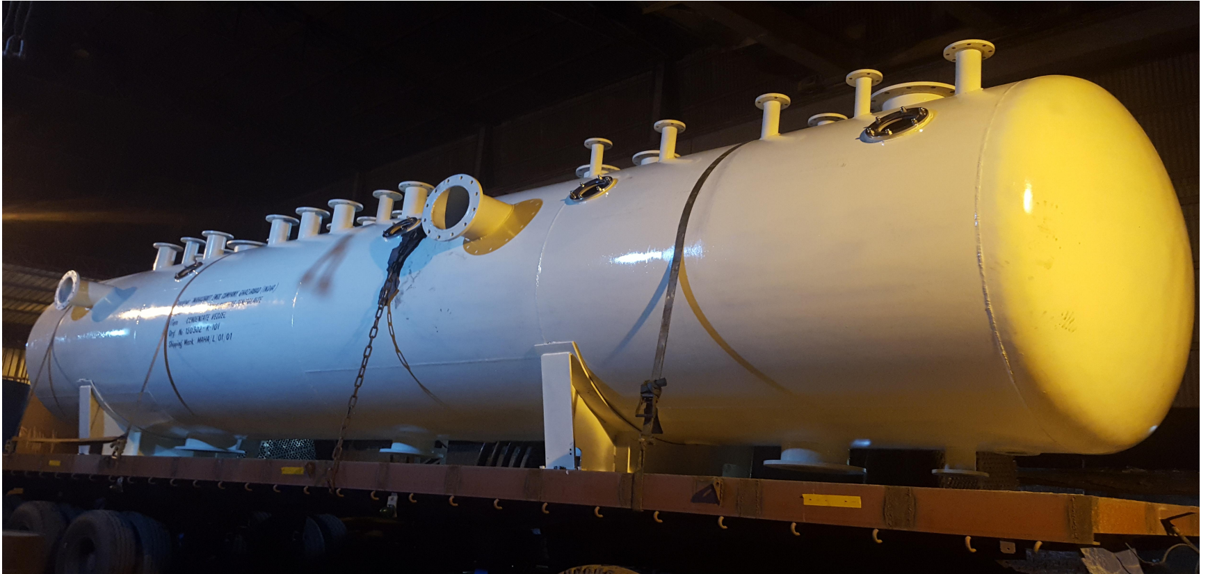
CONDENSATE FLASH VESSEL
